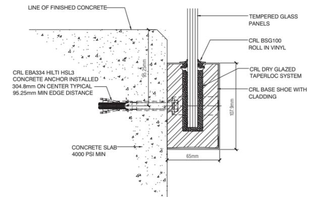
Steel Tube Substrate Typical Surface Mount Detail
