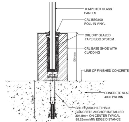
Concrete Substrate Typical Fascia Mount Detail
